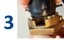
3 Align the replacement dial properly into its designated orientation (poke yoke) and press it down straight into the body — avoiding pivoting it as it can displace the seal.
