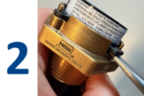
2 Tweak the dial out of the body by using a flat screwdriver underneath the dial flats
