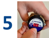
5 Press the button — it should read "Lo"
