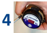
4 Fix the dial with the 2 screws
