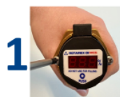
1 Remove the two screws fixing the dial to the body
